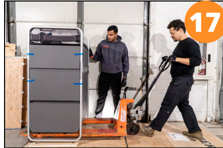
While one person is jacking up the WAZER Pro, the other person keeps the machine stable
