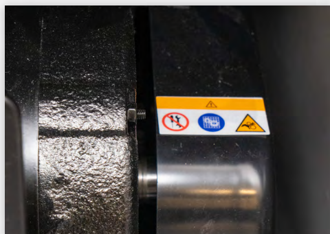
This label warns you entanglement damage exist with revolving pulleys. Keep the Belt Guard in place during WAZER Pro operation.
