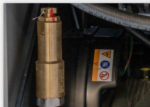
This label warns you entanglement damage exist with revolving pulleys. Keep the Belt Guard in place during WAZER Pro operation.
