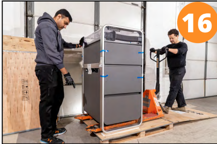
While one person carefully push the pallet jack under the WAZER Pro, the other person helps and ensure pallet jack stays on the pallet
