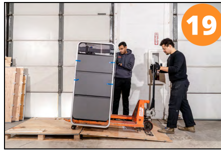
Pull the pallet jack and move WAZER Pro off the pallet. It is vital to have the other person keeping the machine stable in this step
