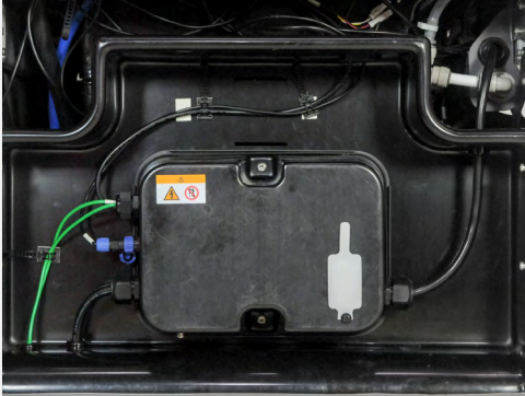
This label warns you of the electrical residual hazards inside the WAZER Pro AC Boxes and warnings against opening them.
