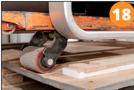
Ensure the pallet jack forks support the bottom ridge evenly, jack the machine all the way up
