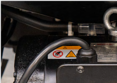
This label warns you of the existence of the high temperature hazard near its proximity.
